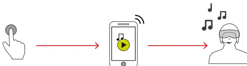
Once the Twins® HF1.0 Dual + HF2.0 Dual is paired to a mobile phone capable of transmitting music through Bluetooth® A2DP, activate music on the phone and it will immediately be heard through the Twins® HF1.0 Dual + HF2.0 Dual device. Music and volume can only be controlled from the phone or device, depending on its features and configuration.
