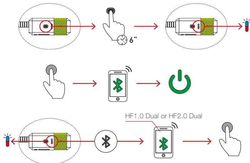
To use the Twins® HF1.0 Dual + HF2.0 Dual, it's necessary to pair it to the Bluetooth® device you wish to connect it to (mobile phone, GPS navigator). While the device is switched off, hold the control button (1b) until the LED indicator (1a) begins flashing in Red and Blue. The mobile phone or GPS navigator will find the device under the name HF1.0 Dual + HF2.0 Dual. Select the HF1.0 Dual or HF2.0 Dual device and, if necessary, enter the access code: 0000.
