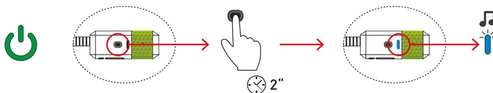
**Switching on:** press and hold the button (1b) for a few seconds until the speakers provides an acoustic signal and the LED indicator (1a) begins to flash in Blue.
