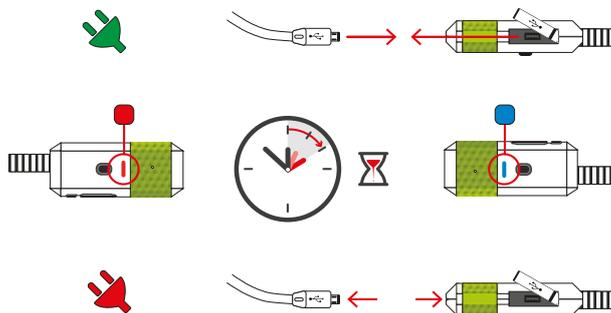
Before using your Twins® HF1.0 Dual + HF2.0 Dual device for the first time, you must charge the device completely. Connect the terminal (1c) to the provided USB charging cable (4) and then connect the cable to a USB charging port. While charging, the red LED light will switch on (1a) and it will change to blue once charging has been completed.
