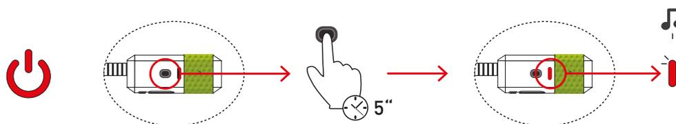
**Switching off:** press and hold the control button (1b) for a few seconds until the speakers provides an acoustic signal and the LED indicator (1a) begins flashing in red before the device powers off.
