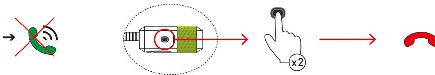
**Rejecting an incoming call:** press the control button (1b) twice, as soon as you hear the acoustic signal for an incoming call.
